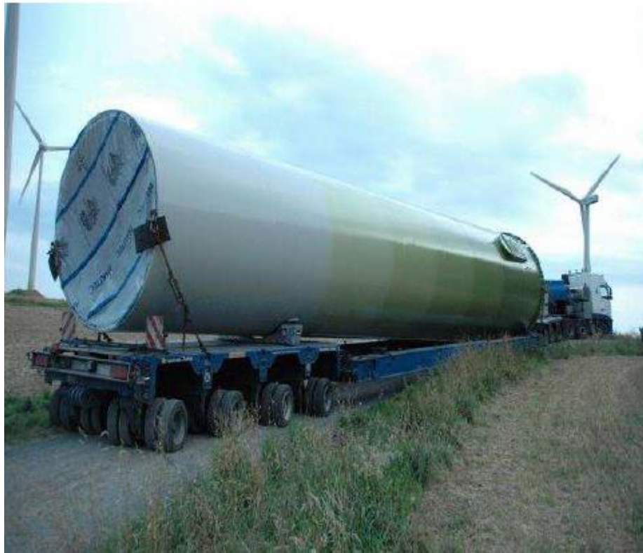
Transportation of wind turbine tower's segments
