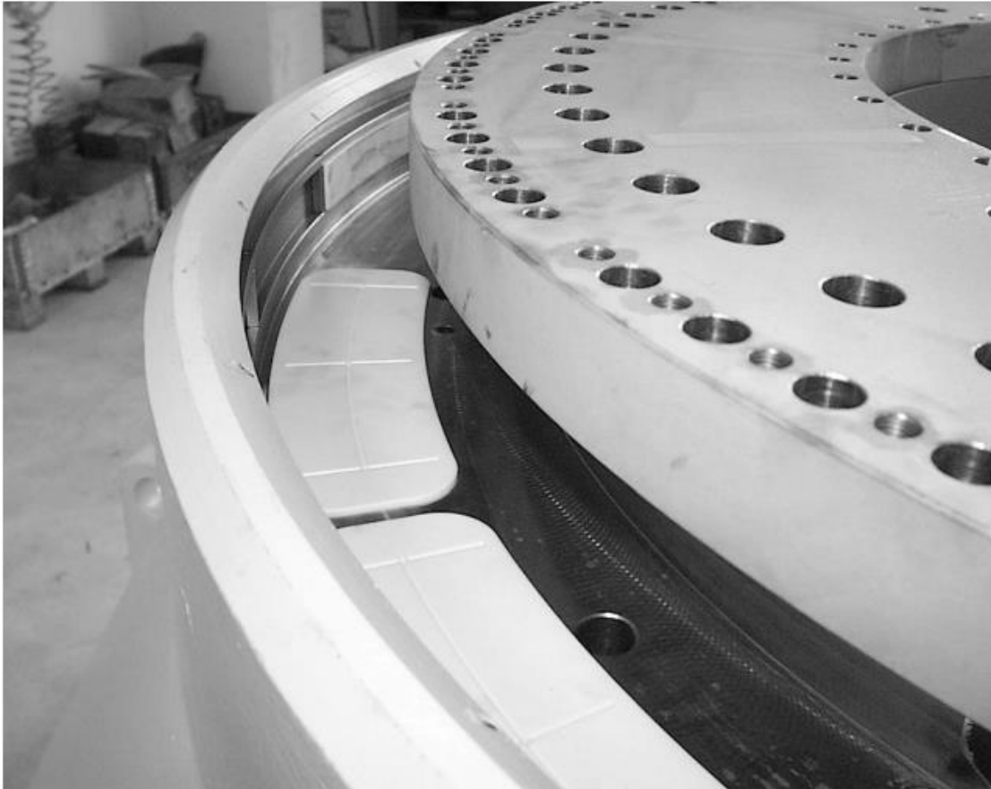
Azimuth friction bearing system of the NEG Micon NM 52
