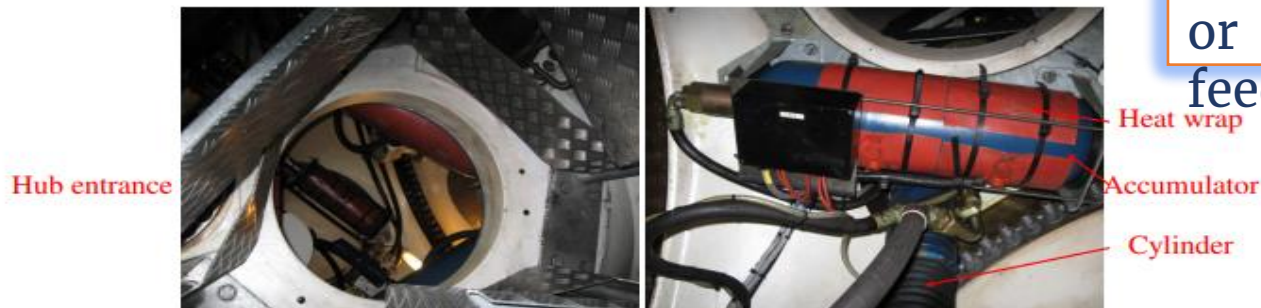
Pitch system components; a hydraulic system in a harsh environment
