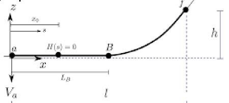
where  $x_0 = L_B - H/(wC_B) \ge 0$ , w is the cable buoyant weight per unit length, E is the cable Young's module, L is the unstreched cable length, A is the cable cross-sectional area, and  $C_B$  is the cable-bed friction coefficient.
