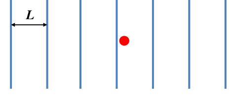
2. Potential flow (H/D < 1) with substantial wave diffraction  $(L/D < 10) \rightarrow$  Froude-Kryloff force + Diffraction force
