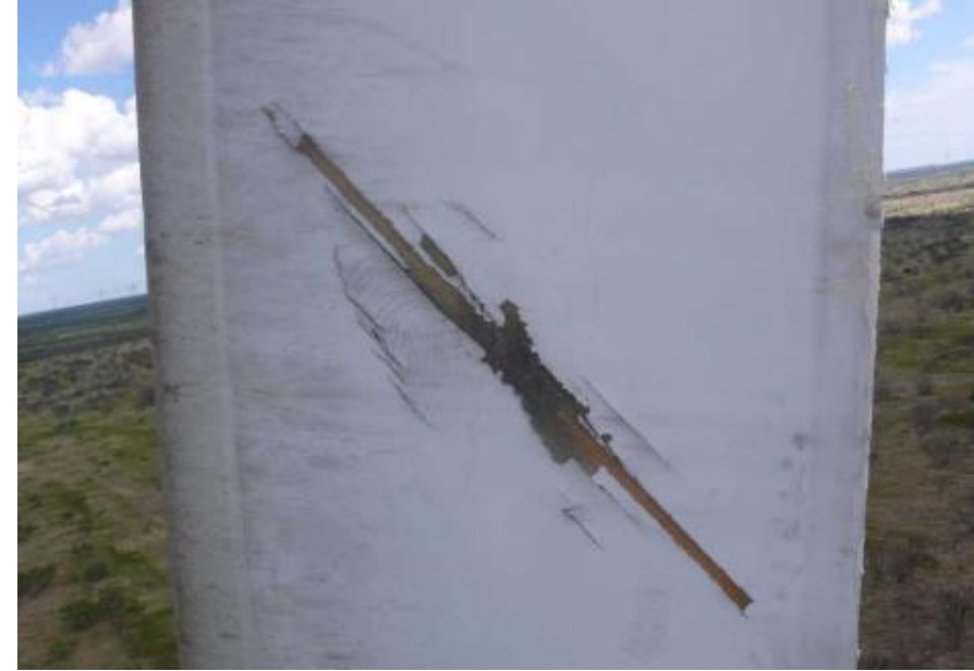
Delamination on the shell at about 2m from the blade tip due to lightning direct strike.
