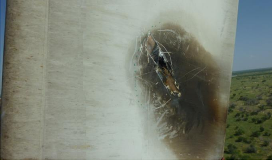
Burn and delamination on the shell at about 3m from the blade tip due to lightning direct strike.
