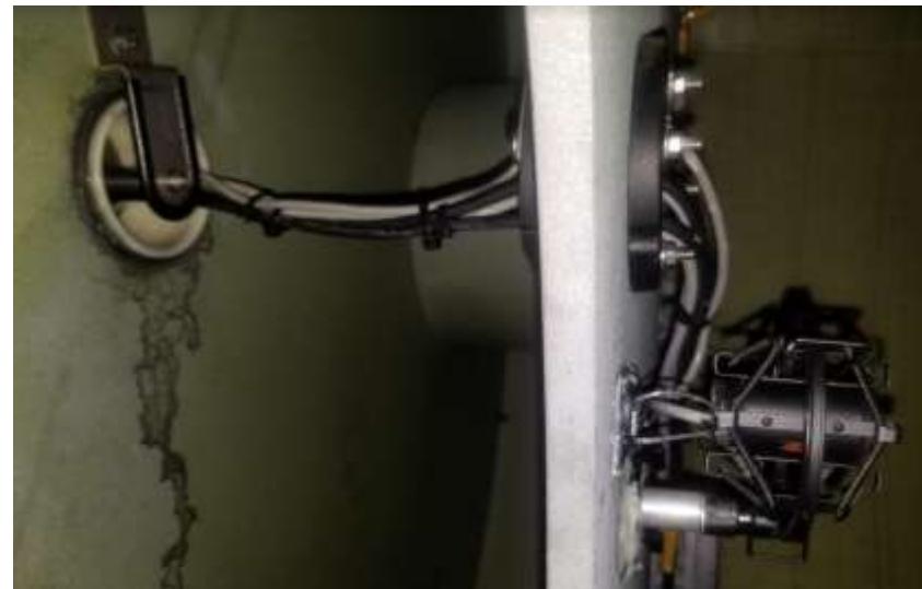
Sensor mounted on the blade bulkhead
