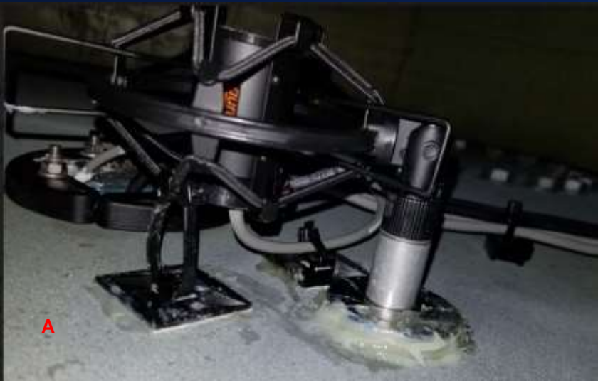
(A) Details of sensor mounting with magnet and epoxy
