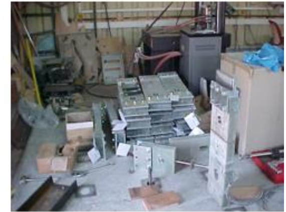
Joint structural part for split blade for tensile testing
