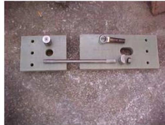
Joint structural part for split blade for tensile testing
