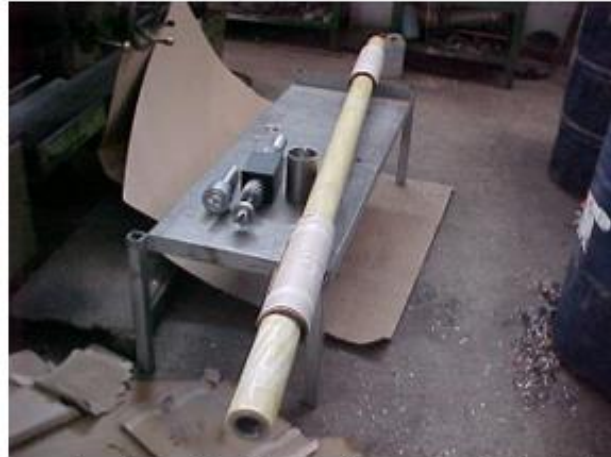
Air brake – blade tip / Internal shaft for stall machines – filament winding
