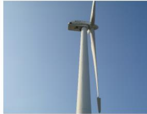
Air brake for stall machines
