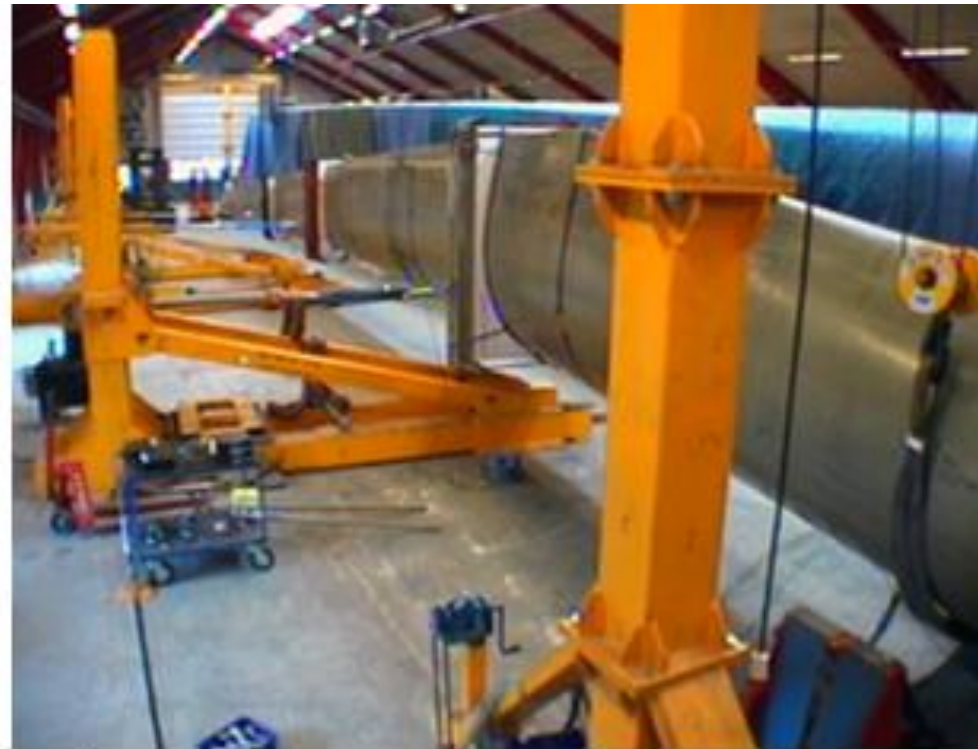
30m split at RISO (Denmark) Lab for testing - year 2002
