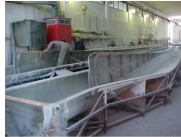
Assembly of shear webs
