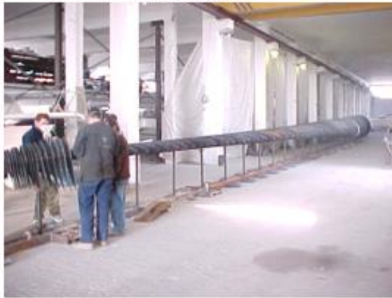
Airfoils have been placed according to the pitch axis
