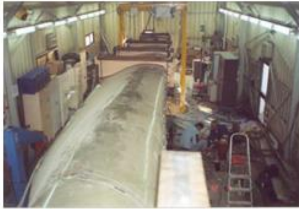
19m blade at CRES lab for testing – year 2000
