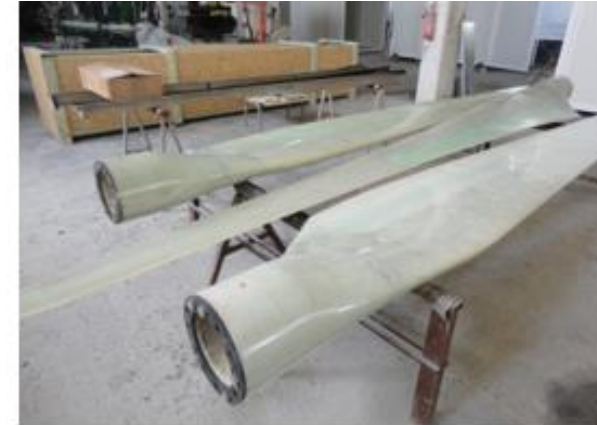
Blades have been demolded
