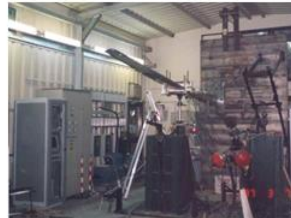
14m and 4,5m blade at CRES lab for testing – year 2002
