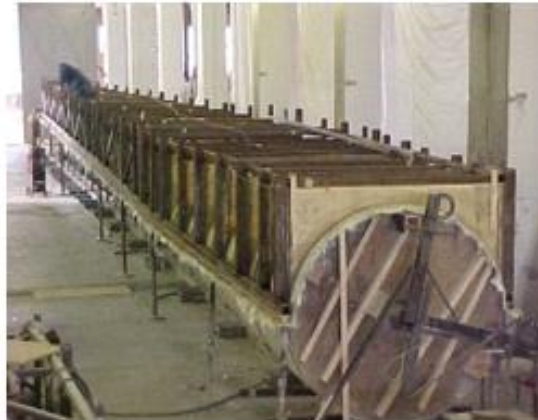
Mold metallic support frame
