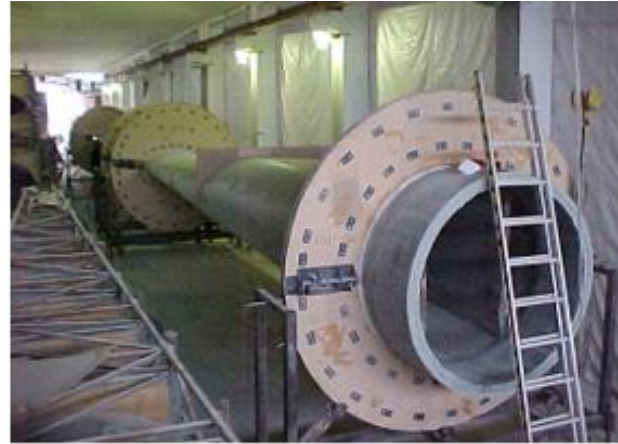
Blades have been demolded
