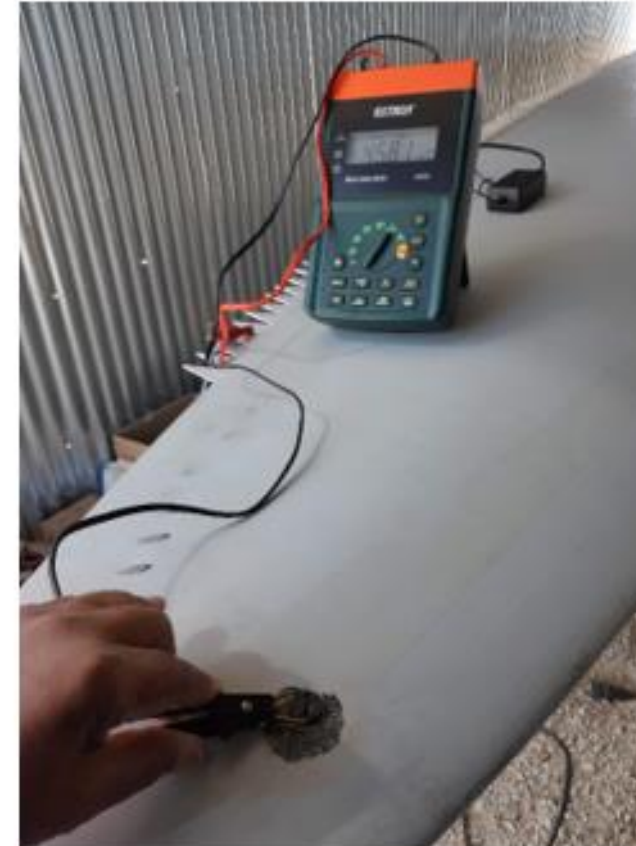
Lightning protection system (LPS), measurement of electrical resistance ( m\Omega s )
