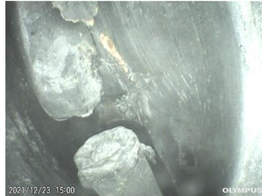
Internal inspection via Endoscope – Broken conductor rod (cable) of Lightning Protection System (LPS of the blade)
