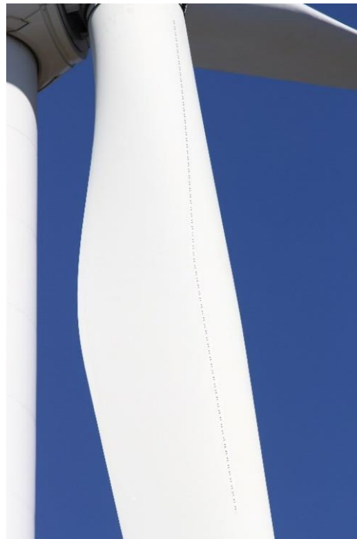
3M Vortex Generators installation at Turkey on 2.5MW (2017), Compblades is VG's certified installer
