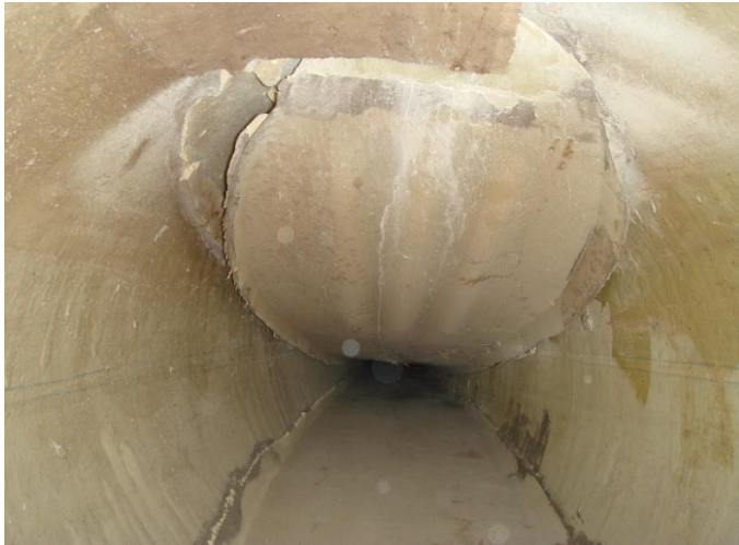
Shear webs were debonded (16m) along the blade skins. Blade was repaired and was in service from 2005 till 2010 (repower).
