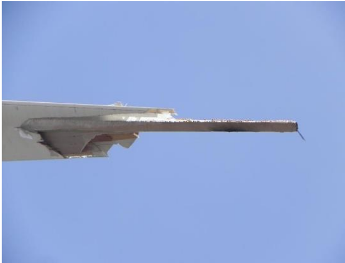
5m skin replacement in 40m blade without moving or turning the blade
