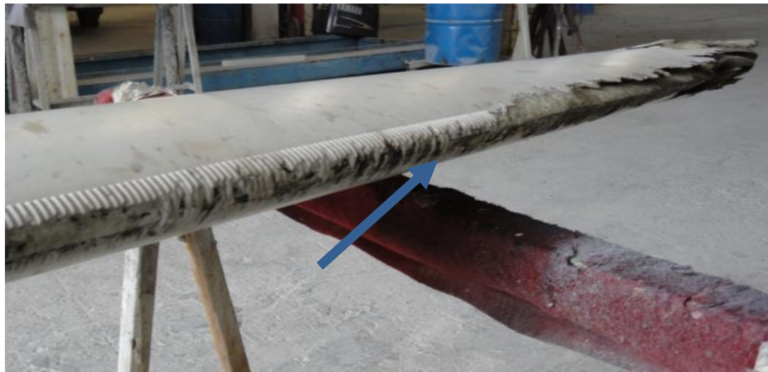
Eroded Blade tip leading edge and destroyed trip strips
