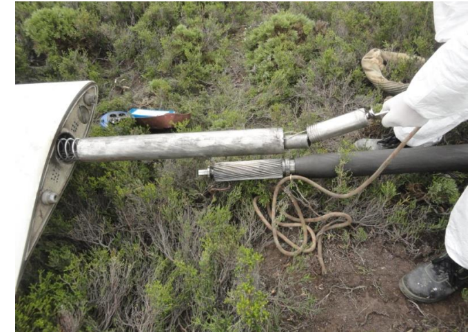
LM 19.1: Broken tube of the blade tip mechanism. A hole is opened on the spar cap to fix the spring end and reconnect the tube for the wire
