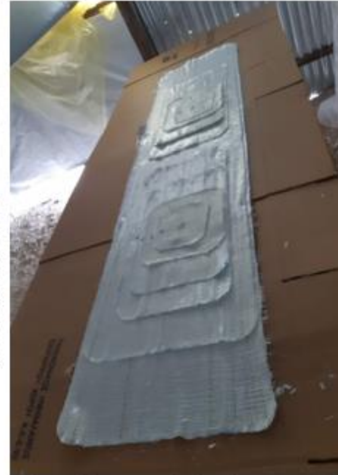
Glass fibers ready for lamination
