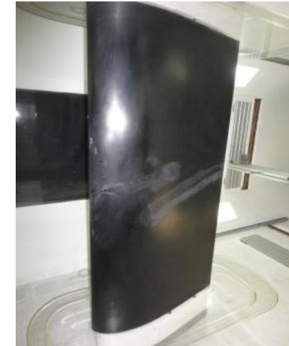
Measuring aerodynamic performance (wind tunnel at NTUA) after leading edge repair - 100% Recover
