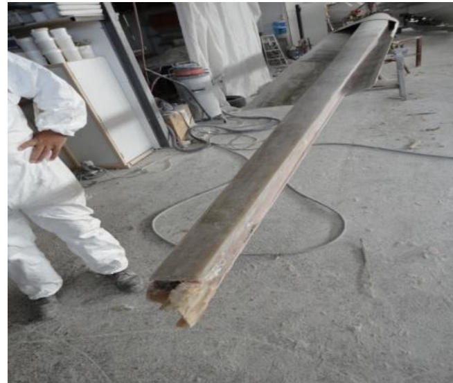
Skins and Spar box repair
