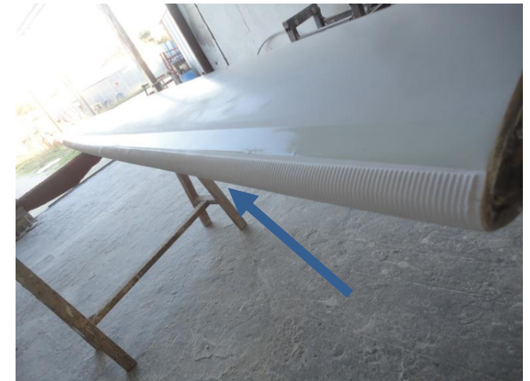
Repaired leading edge new trip strips
