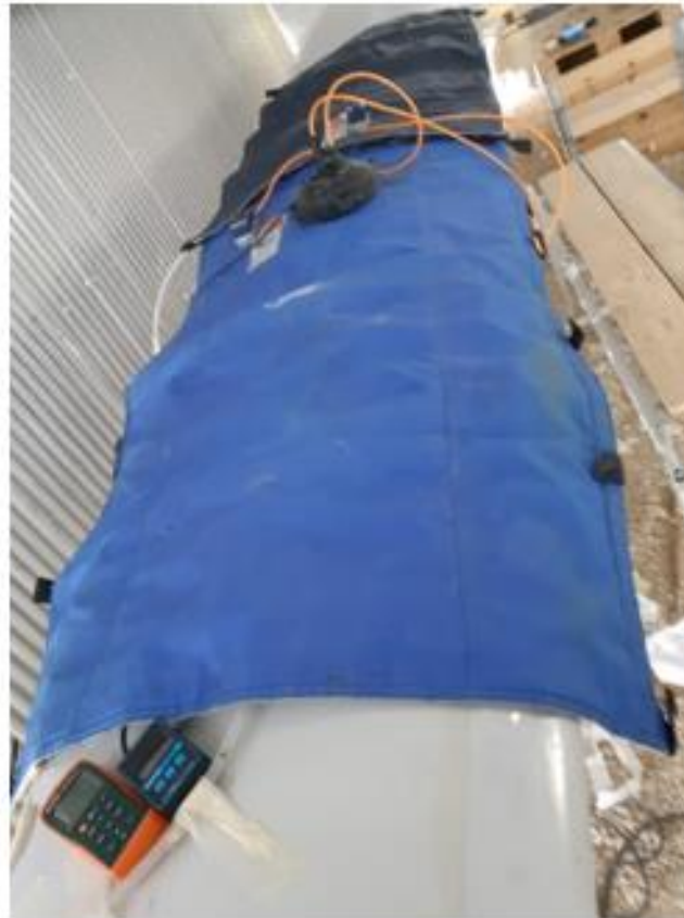
Data logger for curing program via thermocouples and vacuum pressure
