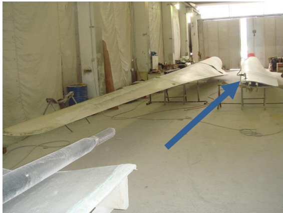
Blade reconstruction: Restoration of the blade in a 7m length.
