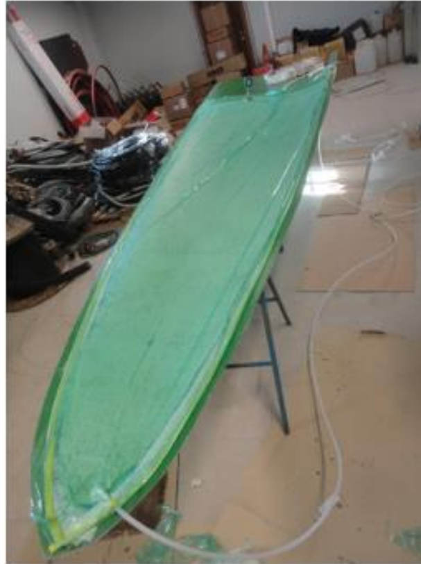
Replacement parts construction via vacuum bagging
