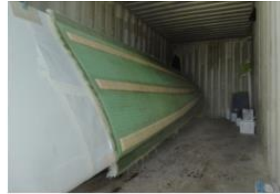
4m mold for the construction of replacement parts
