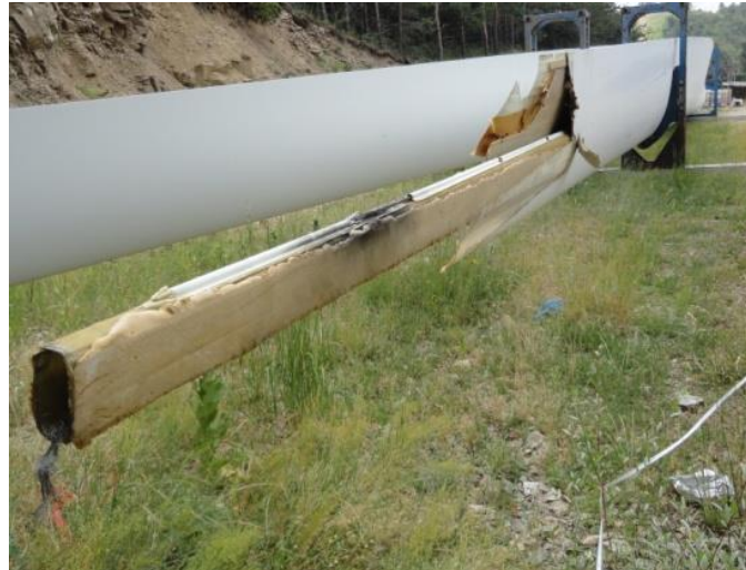
5m skin replacement in 40m blade without moving or turning the blade
