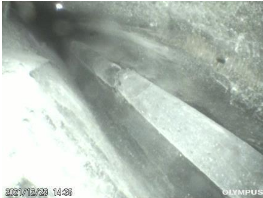
Internal inspection via Endoscope – Broken conductor rod (cable) of Lightning Protection System (LPS of the blade)
