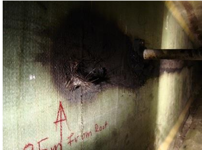
Burnt shear web from lightning and plastic tubular steel-rope container. Shear web was repaired, and plastic tube was replaced
