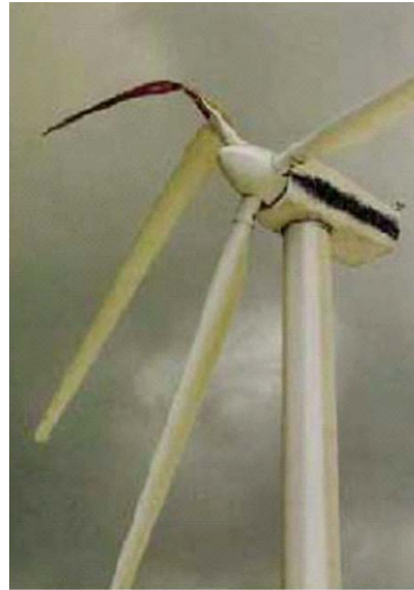
Ruptured blade due to gradual cracking after Lighting strike
